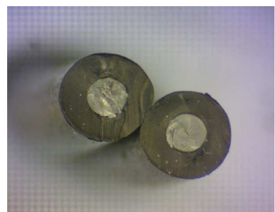
Figure 4. Poor quality termination finish
