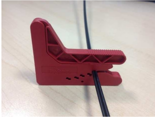
Figure 1. Cutting POF cable on the 'open' slot
